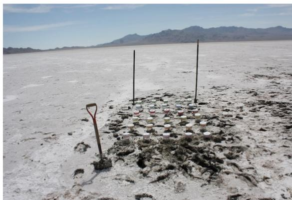
**Figure 4:** In Situ perchlorate reduction field experiment.
